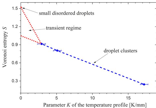
**Fig. 3** Effect of local heating of water surface on ordering the levitating droplets
