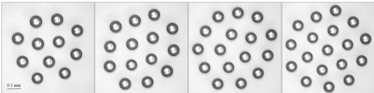
**Fig. 6** Typical small clusters of nearly identical droplets. Clusters of 11, 14, 16, and 18 droplets (from left to right)
