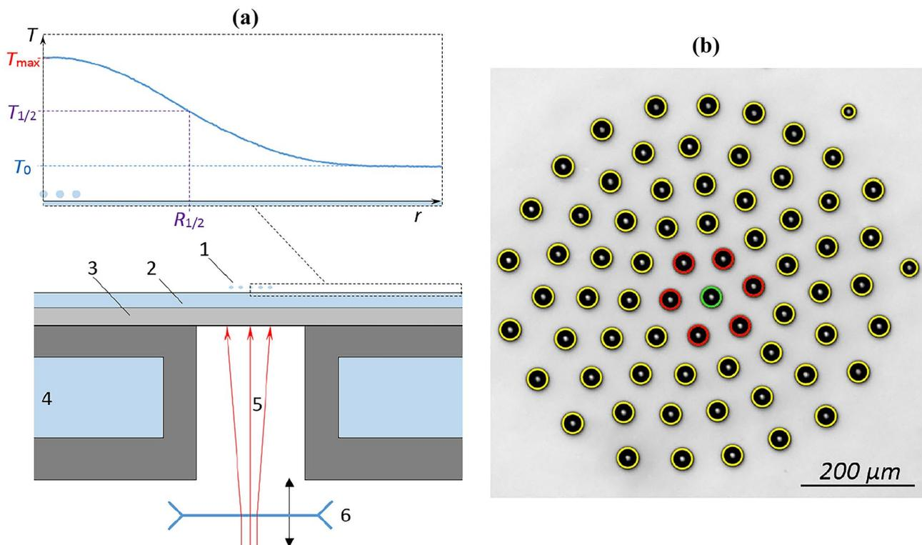
**Fig. 1** **a** The schematic of local laser heating of water and **b** the top view of droplet cluster
