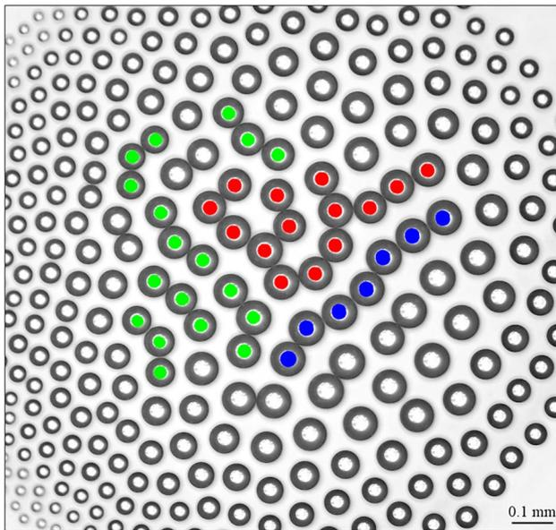
**Fig. 7** A part of an asymmetric cluster containing growing branched chains of water droplets
